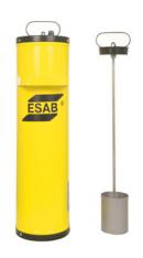
PSE highly portable dry-storage containers ensure that electrodes remain in optimal condition by allowing continued drying or moisture removal until the moment they are used. Simply transfer electrodes from a stationary drying oven or electrode bin and plug in the PSE at the welding station. Only the electrodes needed for the job are exposed while the remainder are stored for continued drying.
